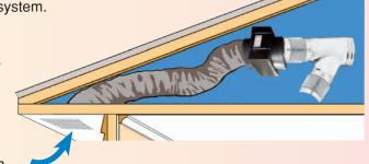
Please note: when the summer feature is working the lounge/warmed room inlet will be switched off via the damper and therefore will not receive the cooled air directly from outside however due to an imbalance of air pressure a natural re-circulation occurs (as shown in diagram no.3).
