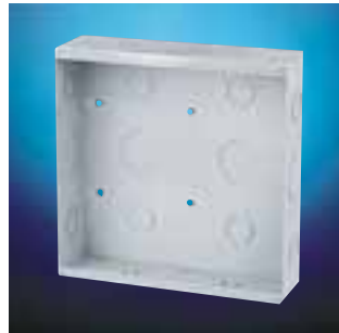
534B16 SWITCH PANEL WALL BOX 16-Way Size: 200mm x 200mm x 60mm deep. 1 earth terminal. Side knockouts: 2 x 38mm, 4 x 25/21mm. Back knockouts: 2 x 38mm, 4 x 25/21mm.
