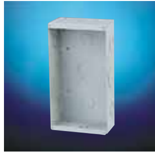
534B8 SWITCH PANEL WALL BOX 8-Way Size: 108mm x 200mm x 60mm deep. 1 earth terminal. Side knockouts: 2 x 38mm, 4 x 25/21mm. Back knockouts: 11 x 38mm, 2 x 25/21mm.
