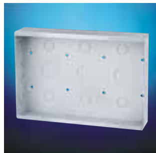
534B24 SWITCH PANEL WALL BOX 24-Way Size: 293mm x 200mm x 60mm deep. 1 earth terminal. Side knockouts: 2 x 38mm, 4 x 25/21mm. Back knockouts: 3 x 38mm, 4 x 25/21mm.
