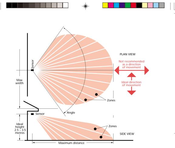
Each zone is constantly monitored by the sensor. When a person or other heat source enters any zone, the level of infra-red radiation in that zone increases.
