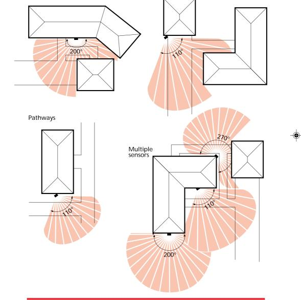
Position the sensor so your normal direction of movement is ACROSS the PIR Zones.
