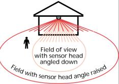
The key to successful operation of any PIR sensor is choosing the correct location. The greater the field of view, the greater the chance of nuisance tripping.
