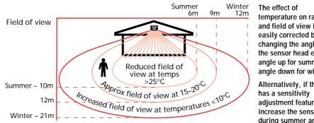
temperature on range and field of view is easily corrected by changing the angle of the sensor head eg angle up for summer or angle down for winter.
